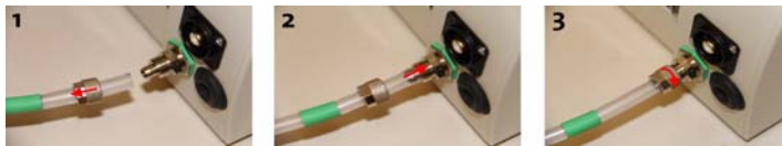
Figure 12 How to connect a tube to a TCU connector. 1 - Slide the nut of the connector onto the tube, 2 - Connect the tube to the connector, 3 - Screw the nut onto the connector.
