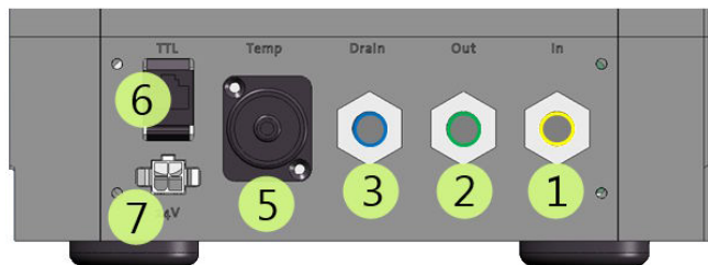
Figure 13 The back panels of the DanioVision Observation Chamber DVOC-0050 (top) and the Temperature Control Unit DVTCU-001x (bottom). The numbers of the connectors / ports are also described in the text above. Connectors with the same number are connected with the provided tubes with the same color-code. 1 - Yellow connectors for water flow into the Temperature Control Unit and out of the Observation Chamber. 2 - Green connectors for water flow out of the Temperature Control Unit and into the Observation Chamber. 3 - Drain connector. 4 - Water overflow connector. 5 - Connectors for the temperature sensor. 6 - TTL ports. 7 - Power connection of the Temperature Control Unit.
